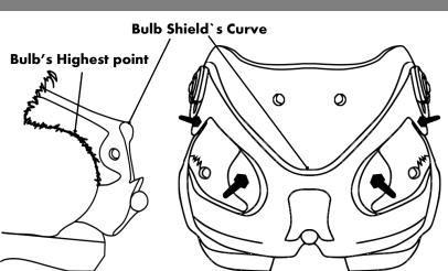
Make sure that the Bulb Shield's Curve surpasses the horse's Bulb's curve highest point.
